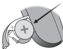
Insert the new battery into the battery drawer. Insert it from above, NOT from the side.
