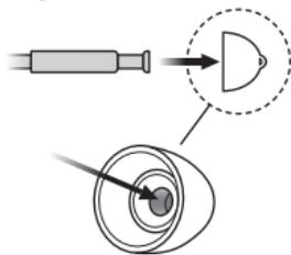
Insert the thin tube exactly into the middle of the earpiece to obtain a secure attachment.
