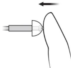
Push firmly to ensure that the dome is fastened securely.
